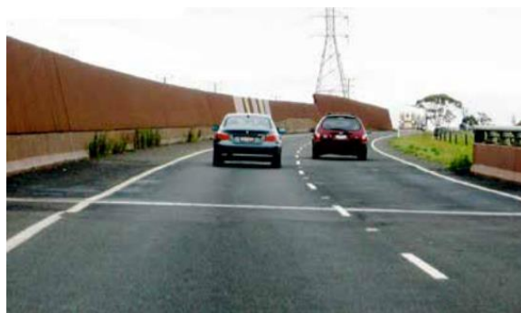
Figure 13. (A) Noise path from source to receiver (Ref. 8), (B) Actual noise barrier to reduce traffic noise.
